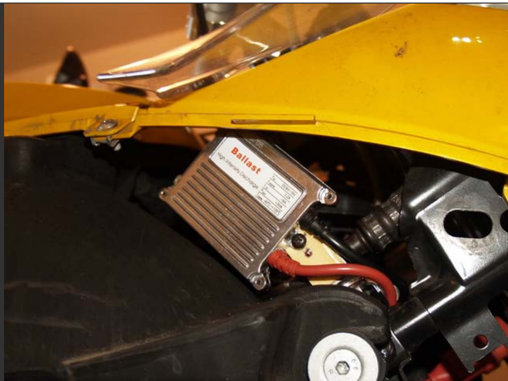
Mounted with double sided tape and a screw.
