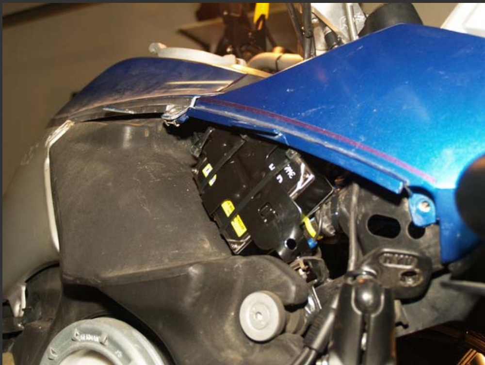
Now you can see it is a tight fit with the beak installed. But it is clean. I added some tie straps to secure the ballast to the mount, and firm it in place as well.
