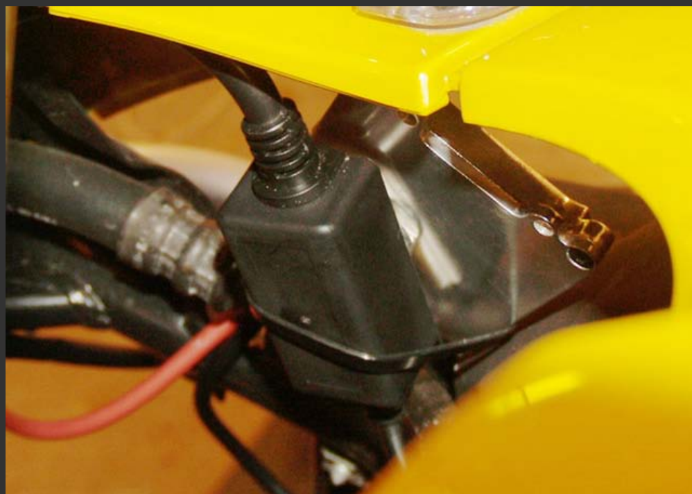
Igniter, zip-tied to the back of the ballast.
