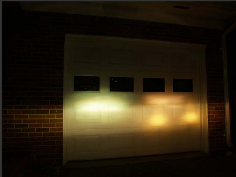
HID (left) and stock, both High Beams, with yellow FF50s on the right.
