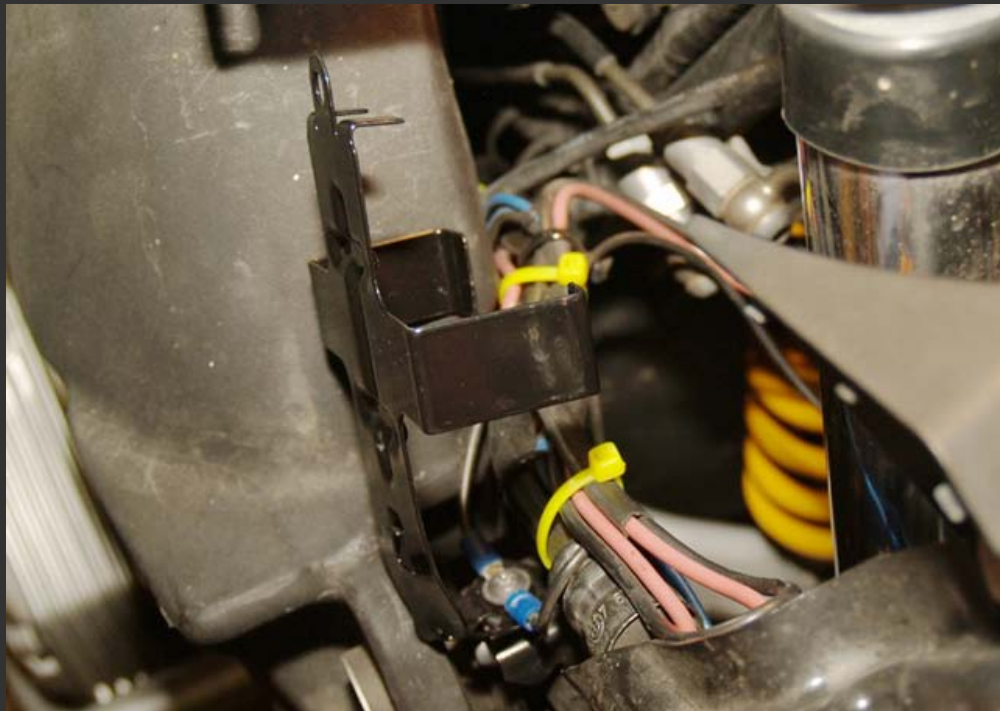
Here is the right ballast mount. You can see it went to the screw holding the oil line.
